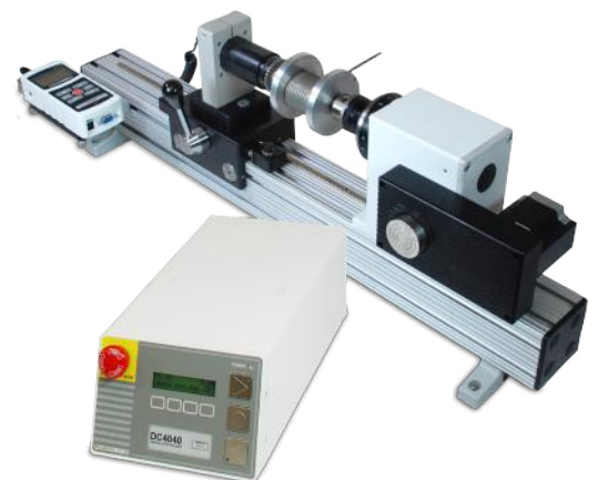
^ The TSTMH-DC is shown in a torsion spring test, with a Series R50 torque sensor and M5i force/torque indicator
