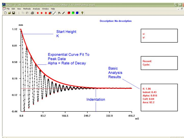
The user can view the graphical display and the numerical parameters are calculated automatically and displayed on the screen. The analysed parameters and raw data can be exported into tab delimited text files.
