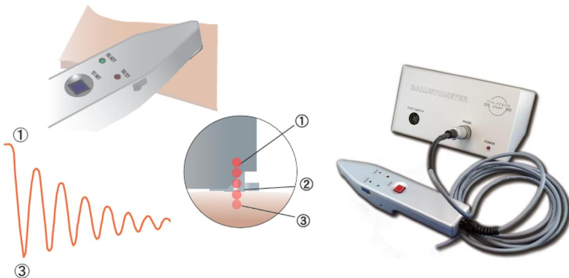
The two main factors that influence the data are the impact force and the dynamic properties of the test site. The user can control the impact force of the stylus using a mechanical switch that is recessed into the Ballistometer probe. At any one setting the elevation and release of the arm generates a constant amount of kinetic energy so that the data is influenced only by the nature of the test site.
