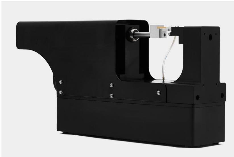
The Dia-Stron LEX820 is a high resolution extensometer developed for the measurement of fine fibres failing at low strain values.
