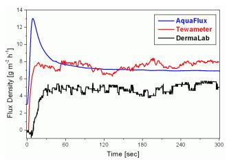
A closed-chamber by itself is no guarantee of performance. Illustrated below is an in-vitro comparison between two different types of closed-chamber instrument. A stable wetcup flux source was used in this test, with 200 repeat measurements per instrument [2].
