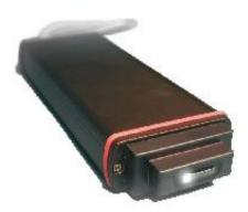
Novel method for investigating translucent materials using hand-held probe. Suitable for use with liquids, emulsions or solids such as skin.
