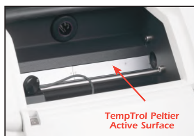
TempTrol heating and cooling Peltier transfer surface
