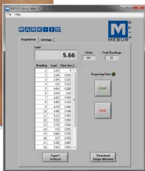
MESUR™ Lite data acquisition software is included with Series 4 gauges
