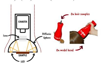
The MAMBO takes advantage of its specific geometry – a diffusive sphere and a stable LED illumination - to always take color measurements in the same and repeatable conditions. Moreover, the color calibrated 12-bit camera enables a high precision comparison of the color of the hair fibers measured and those in its databases without any subjectivity.
